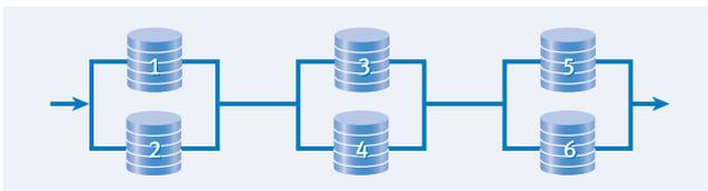
Figure 2. Six HDDs in a RAID-1 configuration
